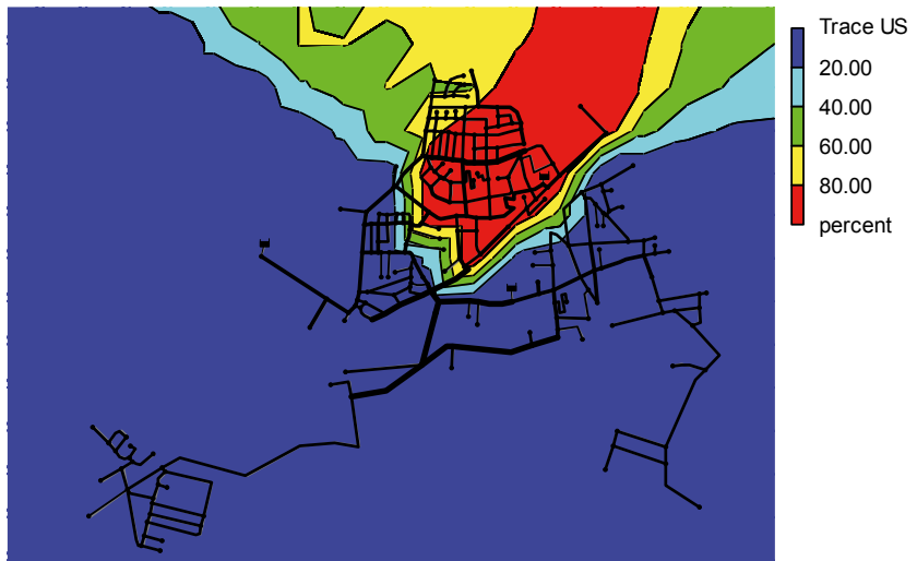
Figure 6. Percentage of water coming from the intake on Płonkowska street relation to the remaining water intakes in the city of Łapy created in the program EPANET on a scale of 1:25 000
