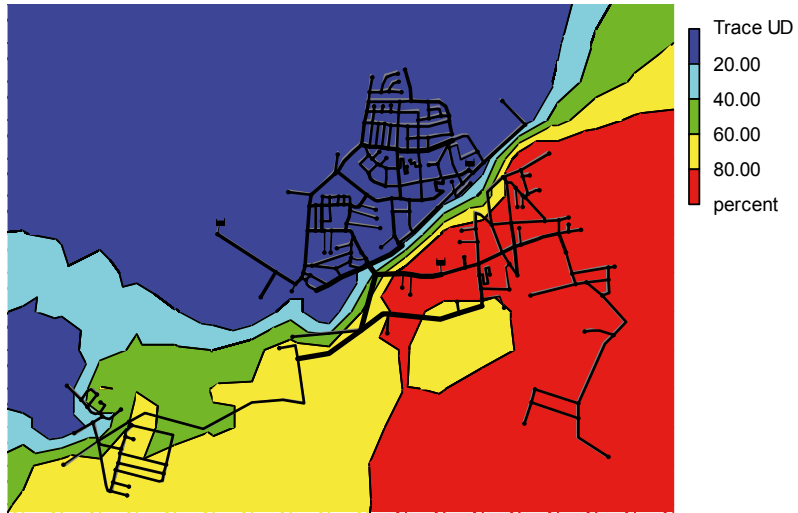
Figure 5. Percentage of water coming from the intake on Długa street in relation to the remaining water intakes in the city of Łapy created in the program EPANET on a scale of 1:25 000
