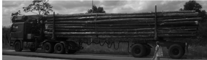
Fig. 8. Transport set five-axle, truck and dolly with different wood assortments: a) Sw 8.8; b) Ls
