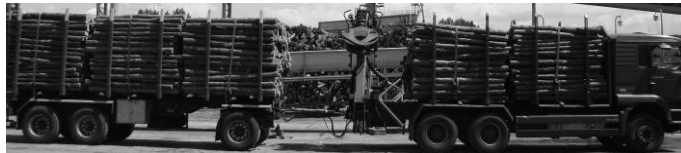
Fig. 6. Transport set truck and semi-trailer with different wood assortments: a) five-axle (3+2) with Ls; b) six-axle with Sw4.4; c) five-axle with Sw8.8; d) six-axle with Sw4.0
