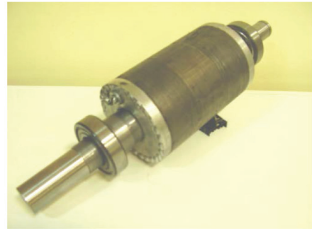
Figure 3. Back in a complete rotor: a) induction motor; b) aluminium cage PMSM
