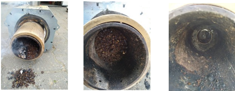
Fig. 4. Burner during firing a mixture of coffee husk pellets and wood pellets at a weight ratio of 70:30. First and second figure from the left: burner clogged with slag (partly and completely); third figure: burner after having been cleaned manually
