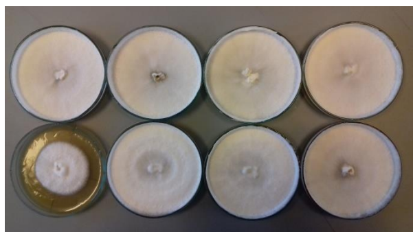
The growth of T. versicolor on a medium with neem essential oil on the 6th day of culture
