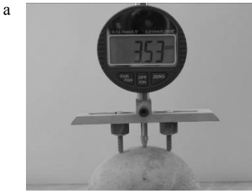
FIGURE 4. Measurement of tuber curvature radius: (a) spherometer, (b) measurement principle
