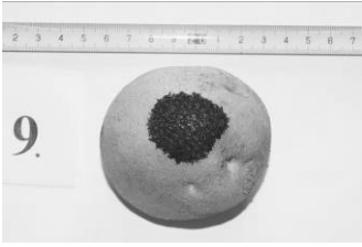
FIGURE 2. Image of the contact area on the potato tuber after impact
