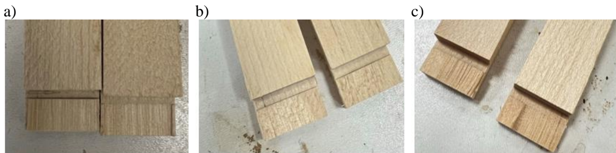
Fig.1. Examples of break zone of the tested samples a) 100 in-wood damage, b) 0% in wood, c) 70% in wood
