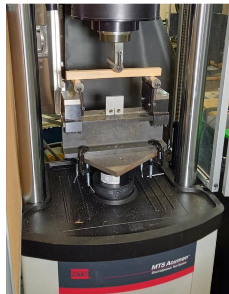
Figure 4. Placing a sample in the MTS Acumen 12 A/T testing machine in accordance with ISO 13061-3
