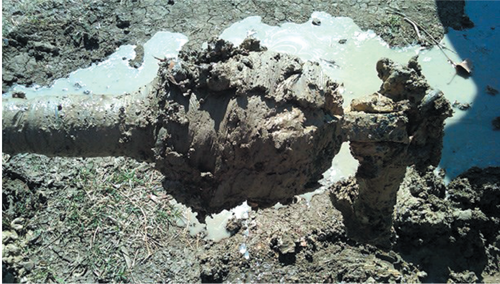
Fig. 1. Drill bit balled up with swelled clays [5]
