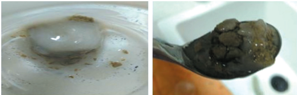
Fig. 8. Condition of the QSE Pellets after swelling test
