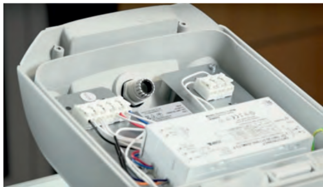
Fot. 6. Sterownik oprawy URBINO LED firmy LUG Light Factory Fot. 6. Lamp holder driver used in the lamp URBINO LED by LUG Light Factory
