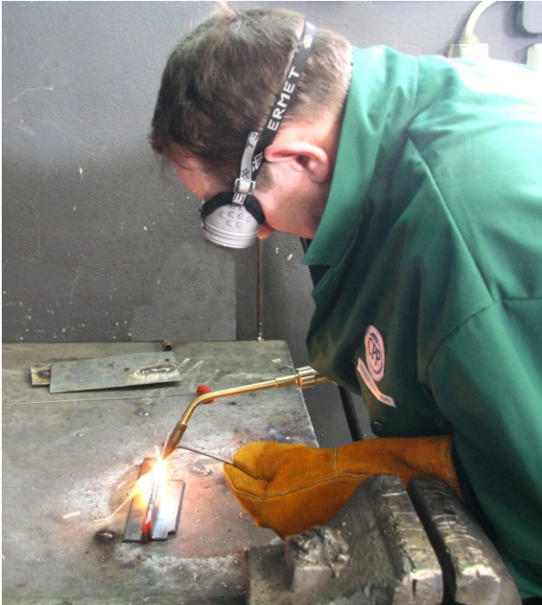
Fig. 3. Example of gas welding
