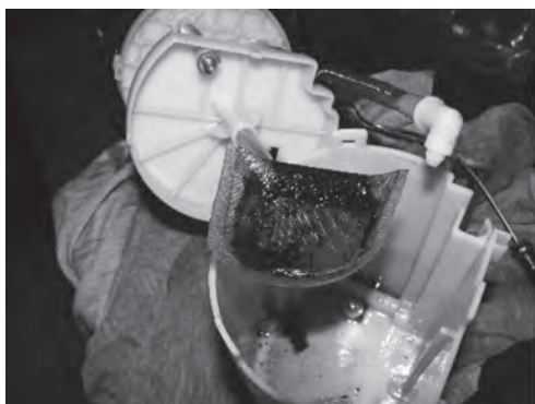
Fig. 2. (Diesel) fuel tank impurities
