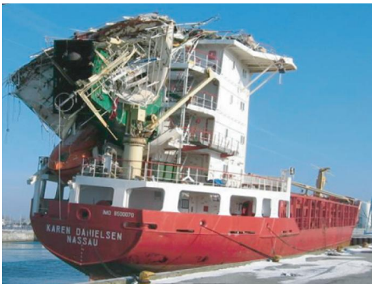
Figure 1. Collision of m/s “Karen Danielsen” with West Bridge in Great Belt (3 march 2005, 1 fatality)
