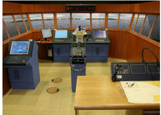
Figure 6. 3D projection visualisation, multi task ship bridge simulator
