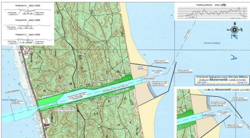
Fig. 2. Design concept of a navigable canal through the Vistula Spit — alternative 1 ‘Skowronki’ [source: www.umgdy.gov.pl/ ]
