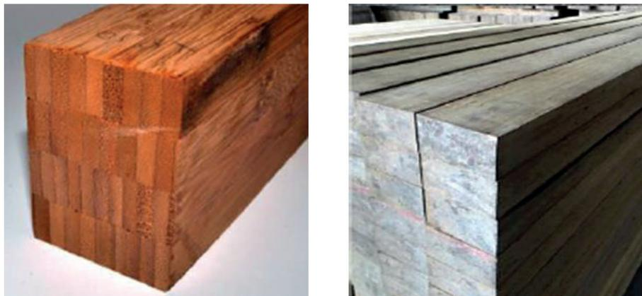
**Figure 5.** (a) Layers of bamboo glued tighter to form laminated bamboo, (b) Bamboo strips compressed together to form bamboo scrimber
