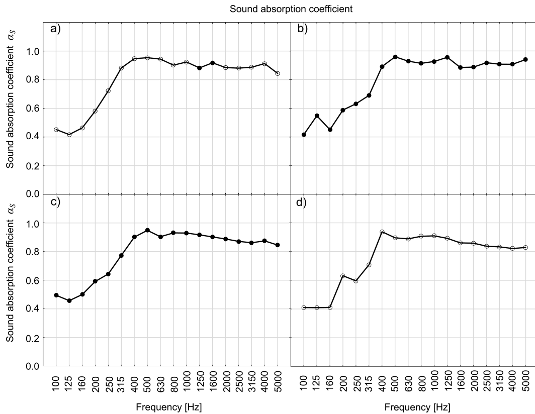
Fig. 7. Exemplary sound absorption characteristics for panels S3: a) at the initial stage, b) after 200 cycles, c) after 450 cycles, d) after 1000 cycles (NOWOŚWIAT et al. , 2016).
