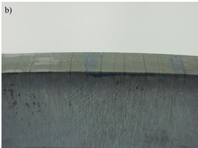
Fig. 4. The damage form of 42CrMo4 steel samples at the end of a static bending test: a) sample views, b) form of cracks on the sample surface
