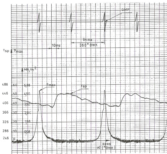
Fig. 2. Time-histories of changes of: exhaust gas temperature, cylinder pressure, and GMP piston position vs. crankshaft rotation angle in single-cylinder four-stroke Diesel engine in two different technical states [Rutkowski, 1976]: a) reference state – full technical ability, b) state of partial technical ability – after introducing engine combustion chamber leakiness (compression pressure decreased from 3,53 to 3,13 MPa).
