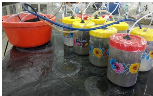
Fig. 1. Microbial fuel cells with different % of agar in a salt bridge
