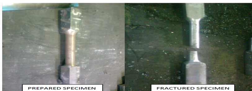
Fig. 3. Test Specimen of structural steel
