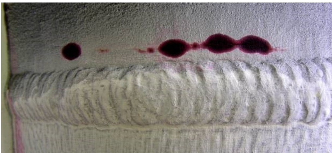
Fig. 7. View of the A1 welded joint from the face side after penetration of the dye penetrant from the inside of the pipe
