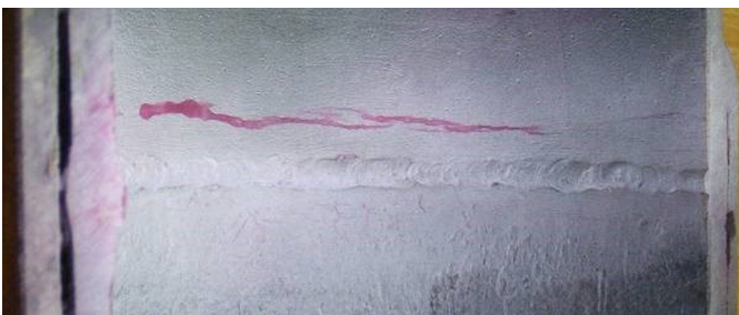
Fig. 9. View of the C1 welded joint from the inside of the pipeline after penetration testing
