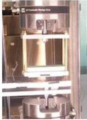
Fig. 4. Measurement test bed with the MTS Bionics 793.00 strength testing machine
