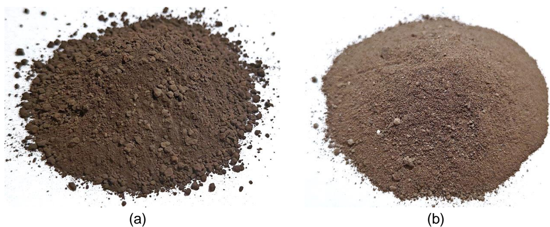
Fig. 1. Waste sludge (a), waste slag (b) before drying
