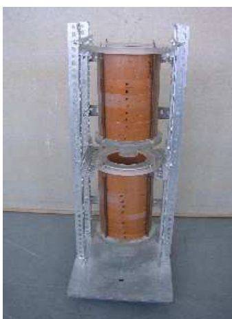
Rys. 1. Mieszalnik laboratoryjny do systemu funnel-flow Fig. 1. Laboratory mixing device used for funnel-flow system
