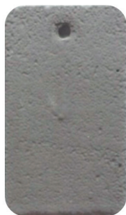
Fig. 1. Sample covered by zirconium – graphite coating to investigations of moisture sorption from surroundings
