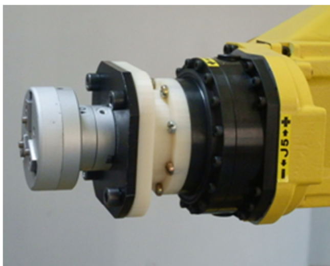
Fig.2. Finished adapter (white) mounted on the robot
