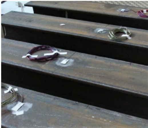
Fig. 3. Rail with strain gauges in place [photo by the authors]
