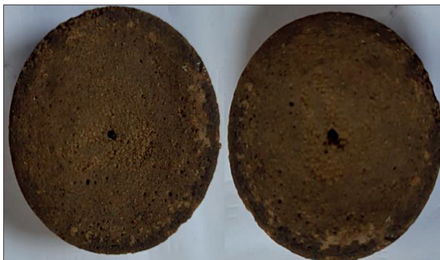
Fig. 4. Pin hole soil samples before and after the test
