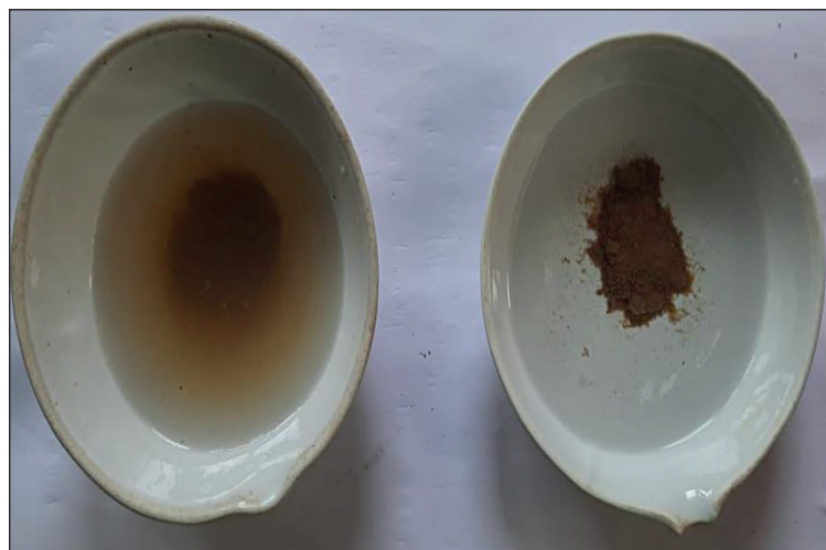
Fig. 11. Crumb test before and after treatment
