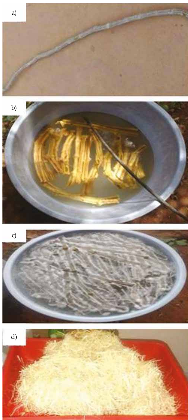
Fig. 1. Fiber extraction: a) full length plant, b) sliced CI, c) CI immersed in water after 3 weeks, d) hewed CI fibers
