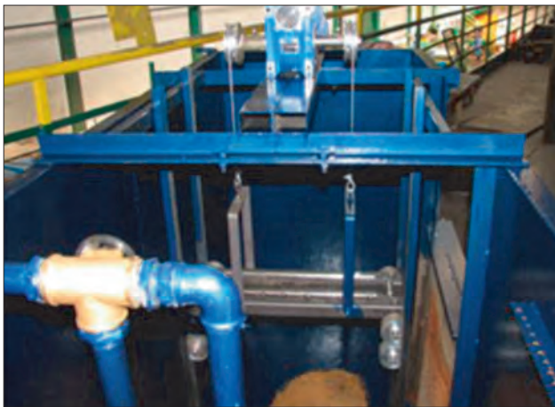
Fig. 1. Equipment for the rail's head hardening process simulation by immersion in polymer aqueous solution
