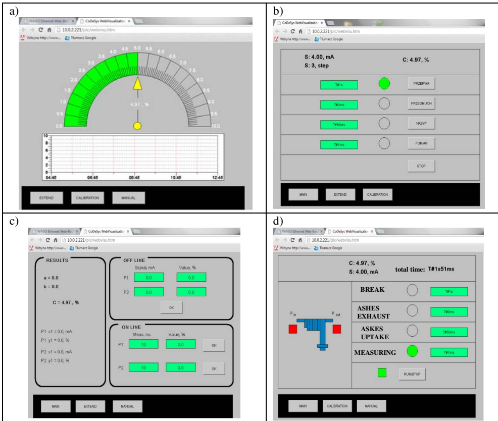
Fig. 4. Windows of the web server in a web browser: a) Monitoring function, b) Measurement service function, c) Calibration function, d) Malfunction service function
