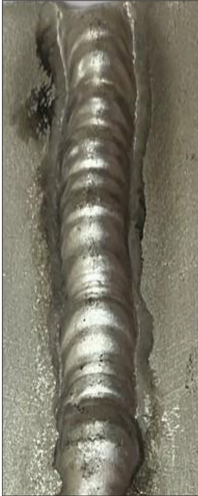
Fig. 2. TIG welding line shape formed in the welding sheet of aluminum piece
