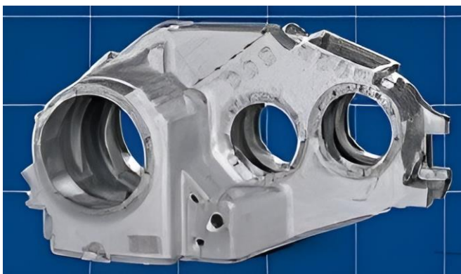
Fig. 1. Test subject – sink rolling bearing housing used in rail vehicles; source: (Thoni Alutec Sp. z o.o., 2021)
