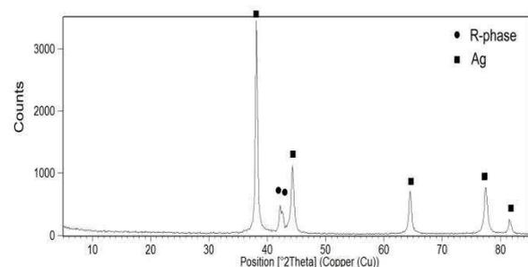
FIG. 3. X-ray diffraction pattern measured for oxidized NiTi alloy covered with Ch/Ag composite.
