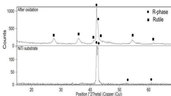
FIG. 1. Comparison of X-ray diffraction patterns measured for as-received NiTi alloy and after its oxidation.
