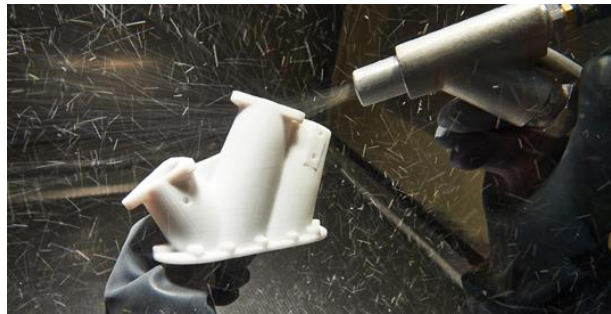
Fig.1. FDM model beat blasting [3]
