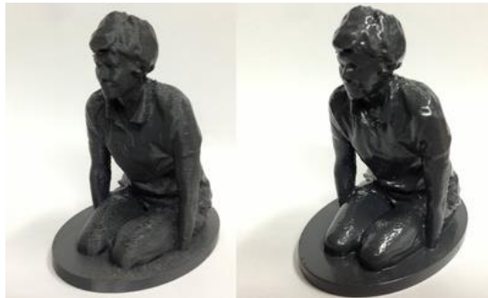
Fig.3. The model smoothed in smoothing station [4]
