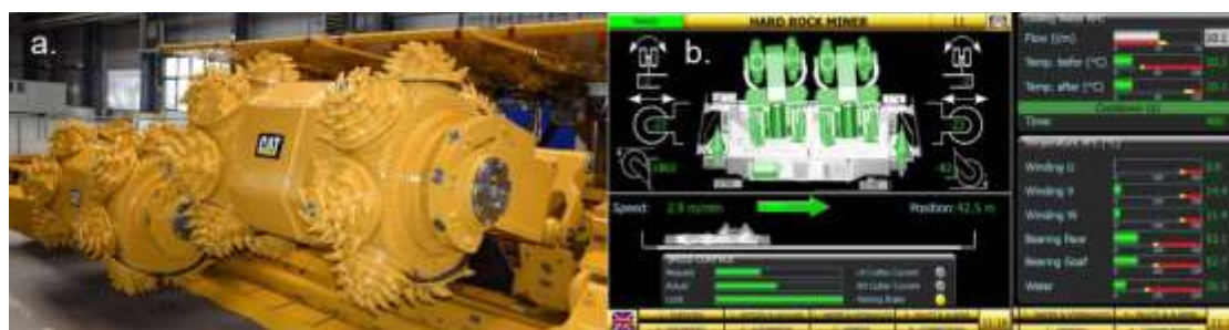
Fig. 9 CAT Rock Straight System: a. view of cutting heads, b. example of a control panel in the operator's cab
