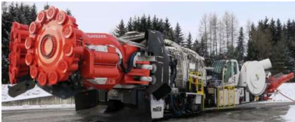
Fig. 7 Sandvik MX650 Rapid Mine Development System
