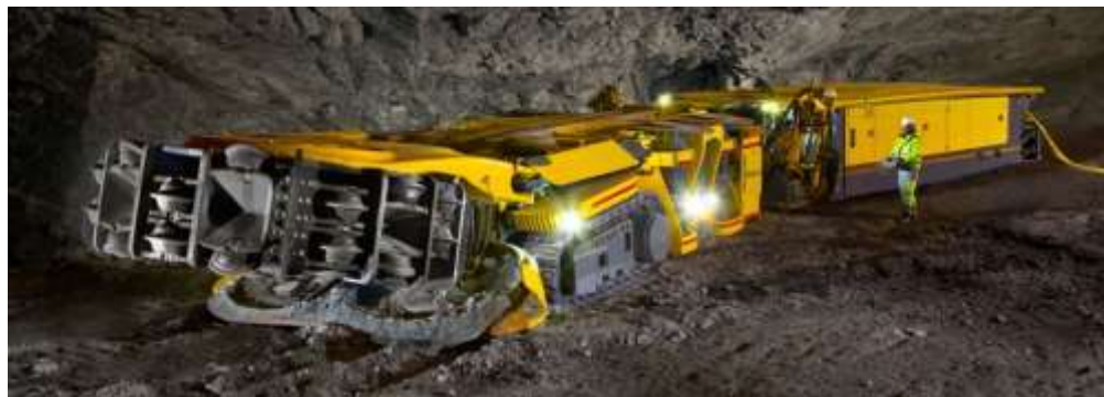
Fig. 3 Epiroc Mobile Miner 22H – in a platinum mine in South Africa
