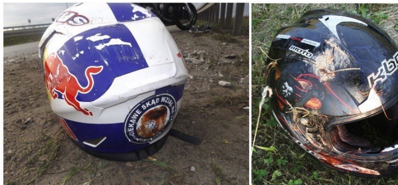
Figure 4. The helmet after hitting a barrier element - broken helmet visor.
