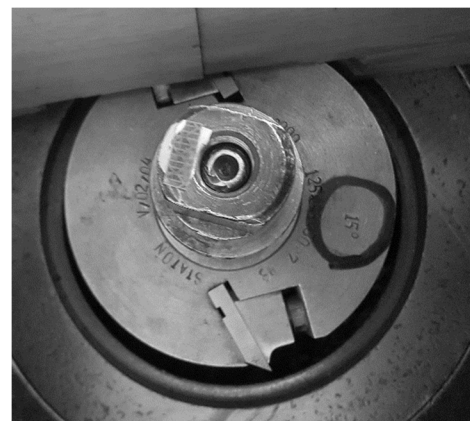
Fig. 7 Milling head with primary clearance angle of 15°
