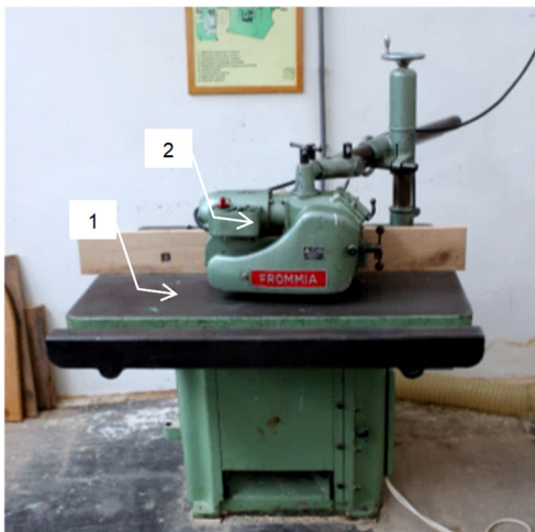
Fig. 4 Spindle miller (1) with feeding mechanism (2)
