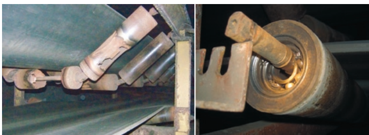
Fig. 9. Examples of premature wear of idlers [10]
