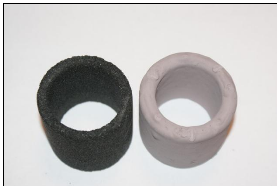
Fig. 2. The core – samples for testing, with and without the deposited coating
