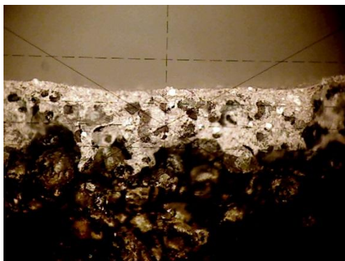
Fig. 12. View of the coating deposited on the core of the moulding sand on the matrix of d_L = 0.34 mm, magnification 30x
