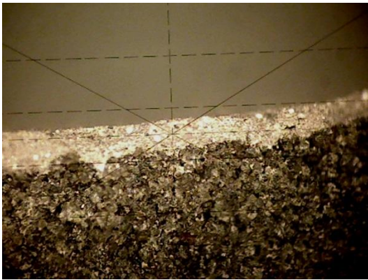
Fig. 10. View of the coating deposited on the core of the moulding sand on the matrix of d_L = 0.20 mm, magnification 30x
