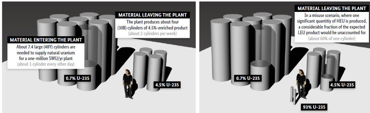
Fig. 7: Uranium entering and leaving a large enrichment plant over a two-week period Source: Glaser, Niemeyer, 2021, p. 101
