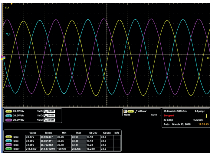
Fig. 25. Idle mode output line voltages measured at constant speed 32.764 rotations per minute
