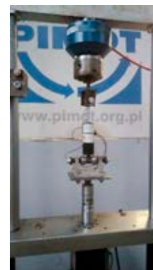
Figure 2. Testing the damper in the test station
