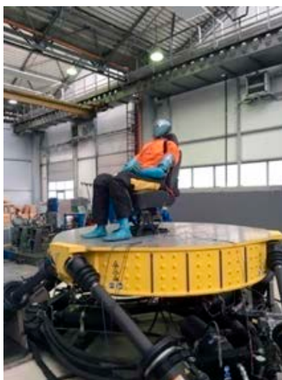
Figure 11. Testing on the M.A.S.T. test station using a dummy
