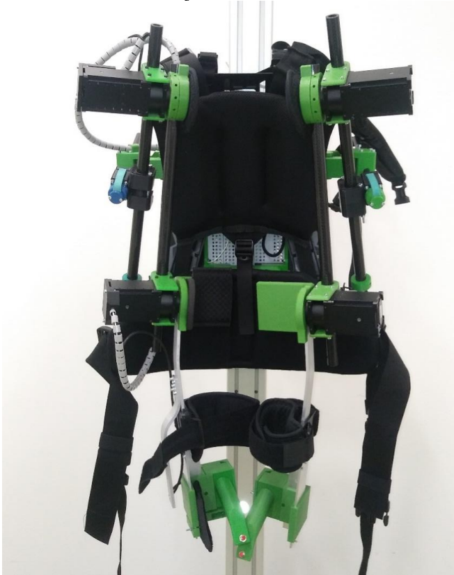
Fig. 1. Functional model of the exoskeleton of the upper limbs (only right hand active)
