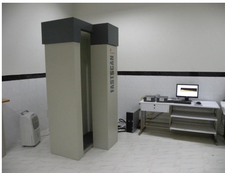
Figure 1. CANBERRA FASTSCAN Whole Body counting arrangement (model 2250).
