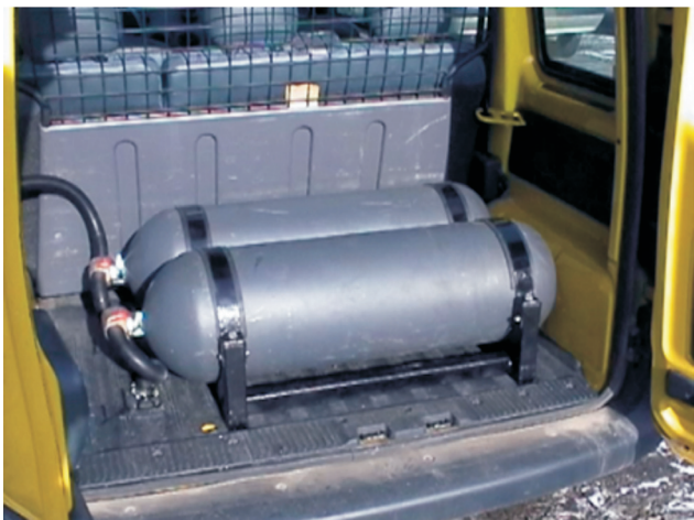
Fig. 4. Steel CNG tanks, p_{max} = 20 MPa Rys. 4. Stalowe butle CNG, p_{max} = 20 MPa
