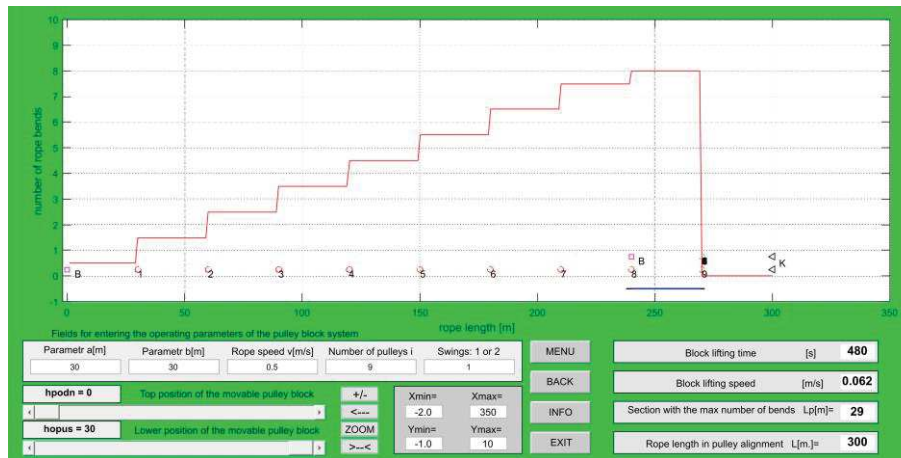
Fig. 7. An example of a diagram for the number of bends of a rope operating in a pulley system for the parameters of the system shown in Fig. 6
