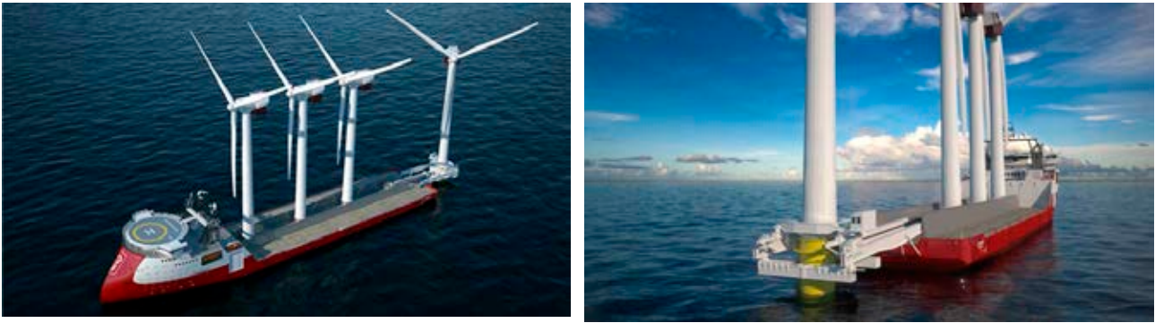
Figure 2. Ulstein Windlifter - the installation system of complete OWT (Douglas-Westwood, 2013)
