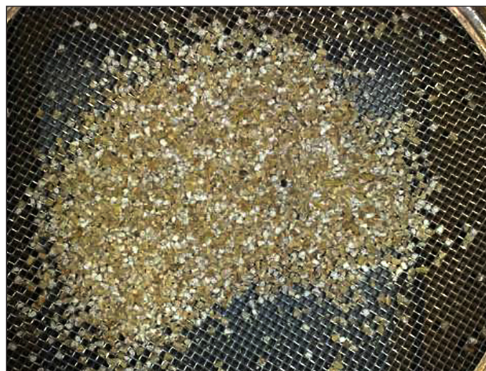
Fig. 5. Exemplary photo of shredded barley accumulated on the screen of a laboratory shaker with square mesh size d_s = 2 mm for peripheral velocity of hammer ends v = 59 \text{ m s}^{-1} , hammer gap s = 15 mm, screen holes d = 5 mm, hammers' angle \alpha = 45^\circ
