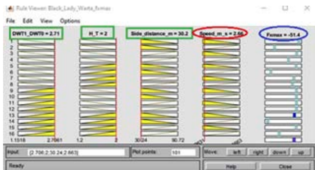
Figure 10. Interface of the SUGENO model with V = 2.66 m/s ( DWT_1/DWT_0 = 2.71 , H/T = 2 , and s = 1B )
