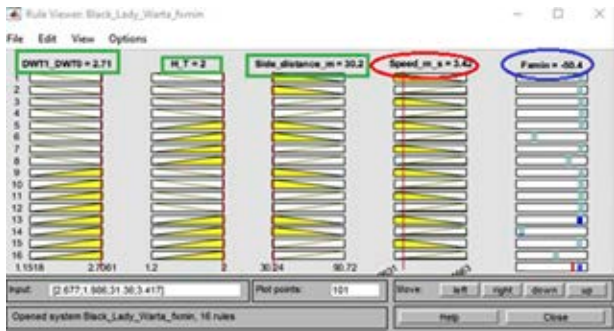
Figure 9. Interface of the SUGENO model with V = 3.42 m/s ( DWT_1/DWT_0 = 2.71 , H/T = 2 , and s = 1B )
