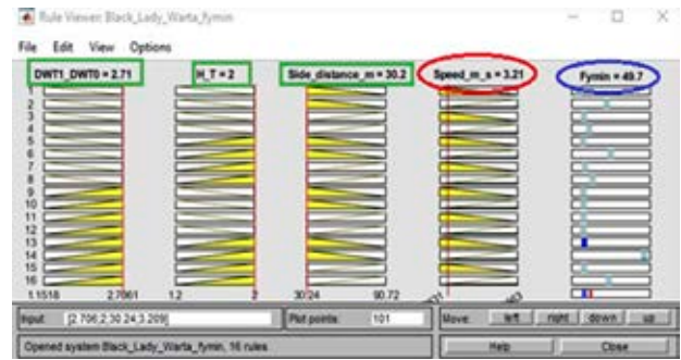
Figure 11. Interface of the SUGENO model with V = 3.21 m/s ( DWT_1/DWT_0 = 2.71 , H/T = 2 , and s = 1B )
